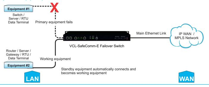
Equipment 1 recovers - Ethernet link automatically reverts and reconnects to Routers, Servers, Switches, RTUs, Data Terminals (any terminal equipment) etc.r-1
