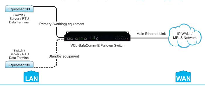
Equipment 1 fails. Ethernet link automatically switches to Routers, Servers, Switches, RTUs, Data Terminals (any terminal equipment) etc.
