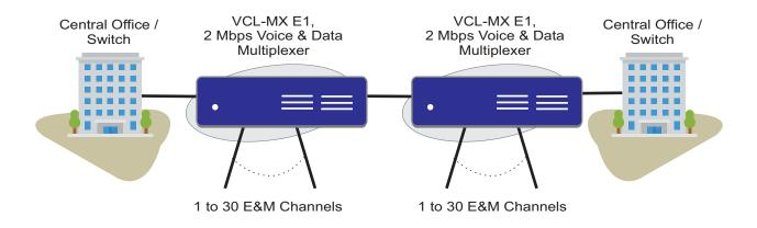
Application # 6: Using in a Subscriber Loop Point to Point or Drop/Insert Application
